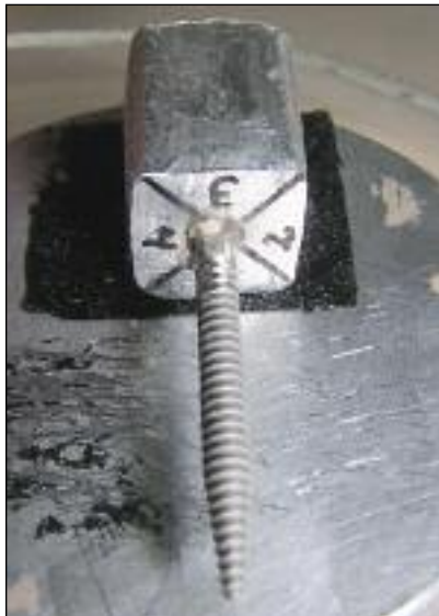
Fig 3 (left and below) Mini-implant on a slide for SEM observation and a diagram showing how all four sides of the implant were examined.
